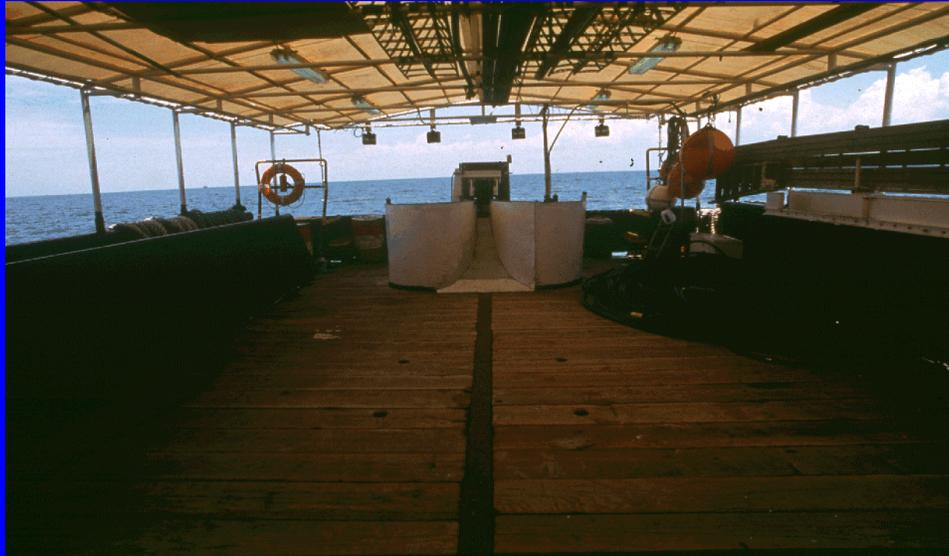
This picture is the back deck of a cable laying vessel showing the "squirter" at center stern for deploying the cables.
