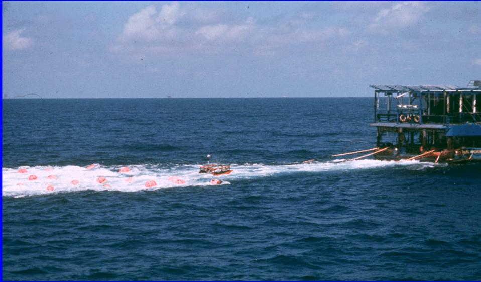
This picture shows the stern of a shooting vessel towing a source array. Notice the GPS antenna positioning the source array.
